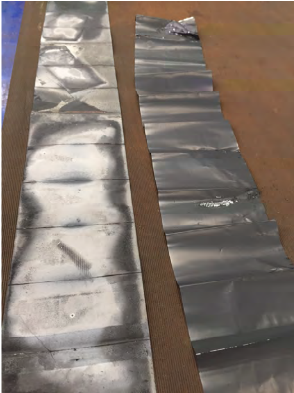
Figure 15: Typical LIB “Jelly Roll” unwrapped showing graphite anode (left) and cathode (right). Underlying copper foil (left) and aluminium foil (right) current collectors can be seen where coatings have been removed during disassembly.
